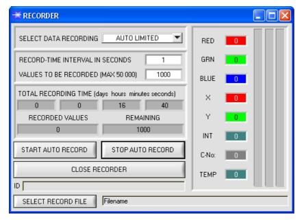
The SPECTRO3-Scope software features a data recorder that allows the saving of RED, GREEN, BLUE, X, Y, INT, C-No: and TEMP. The recorded file is saved to the hard disk of the PC and can then be evaluated with a spreadsheet program.
