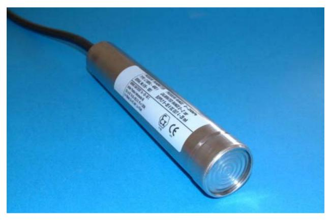
Level transmitter with submersible probe in stainless steel for level measurement in vessels where pressure connection in the bottom of the vessel is not possible or desirable. For exampel pump pits, reservoirs or plastic tanks.
